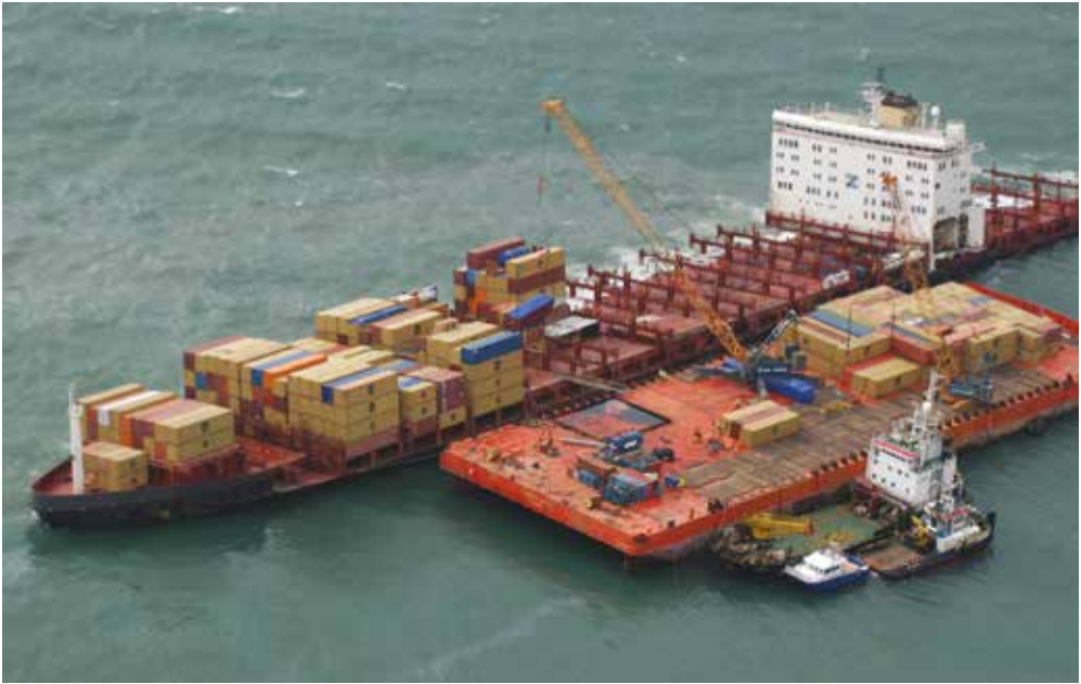
Container ship MSC Napoli suffered severe hull cracks in 2007, probably caused by mis-described container weights
