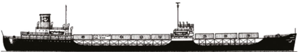
Tanker Ideal-X converted to container ship
